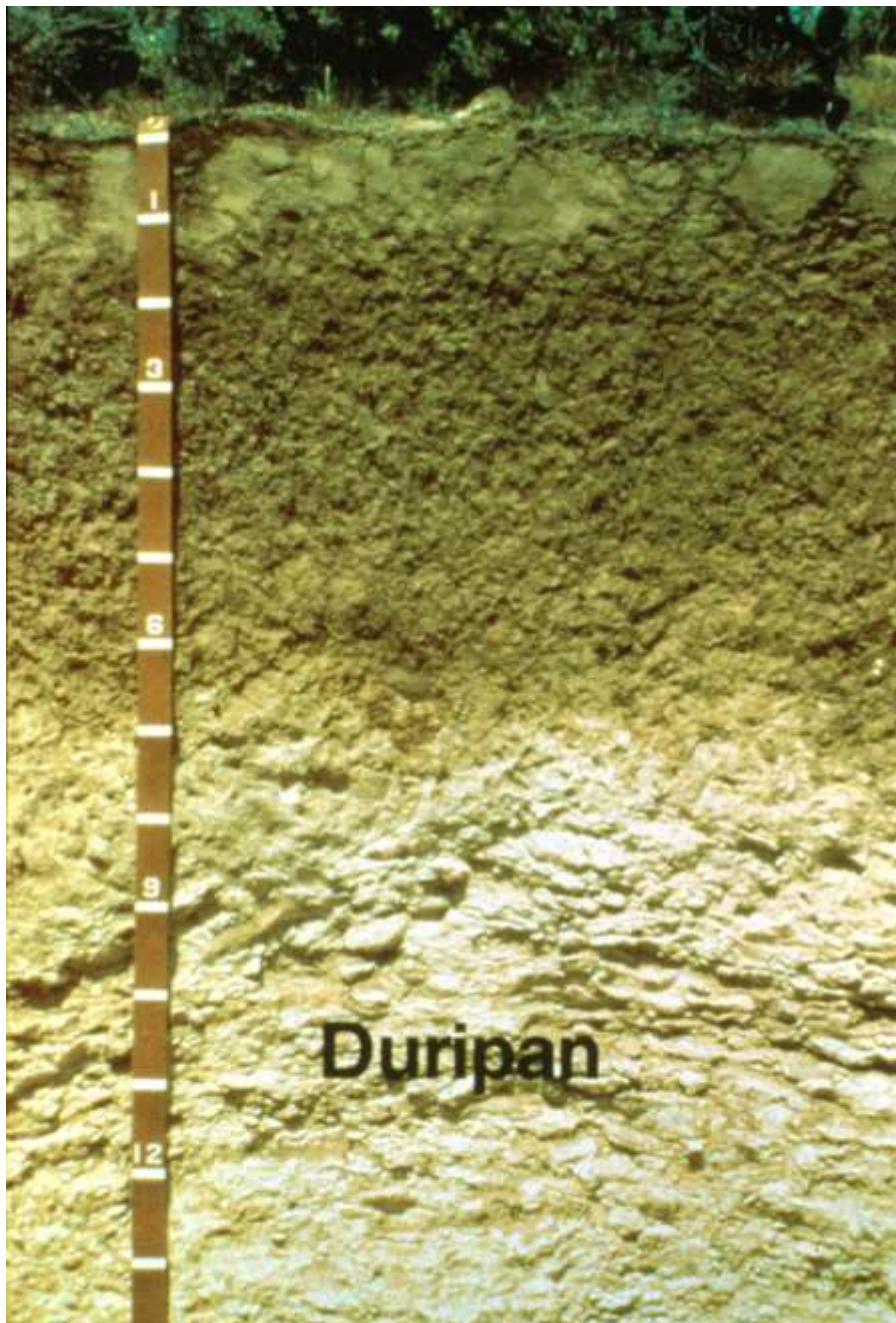
Profile of a Durid (specifically a Haplodurid). The duripan begins at a depth of about 70 cm. Scale in decimeters.
