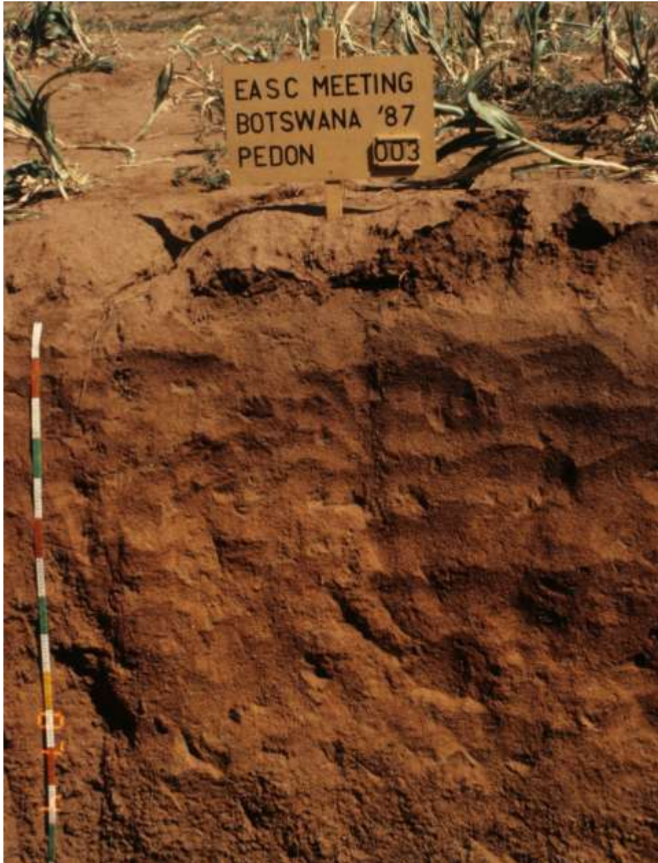
Profile of an Ustalf (specifically a Paleustalf) in Botswana. The soil has a thick clayey argillic horizon. Scale is in decimeters.
