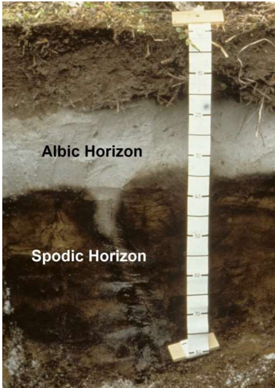
An albic horizon (white) above a spodic horizon (dark brown) in a soil in New Zealand. Scale is in cm.
