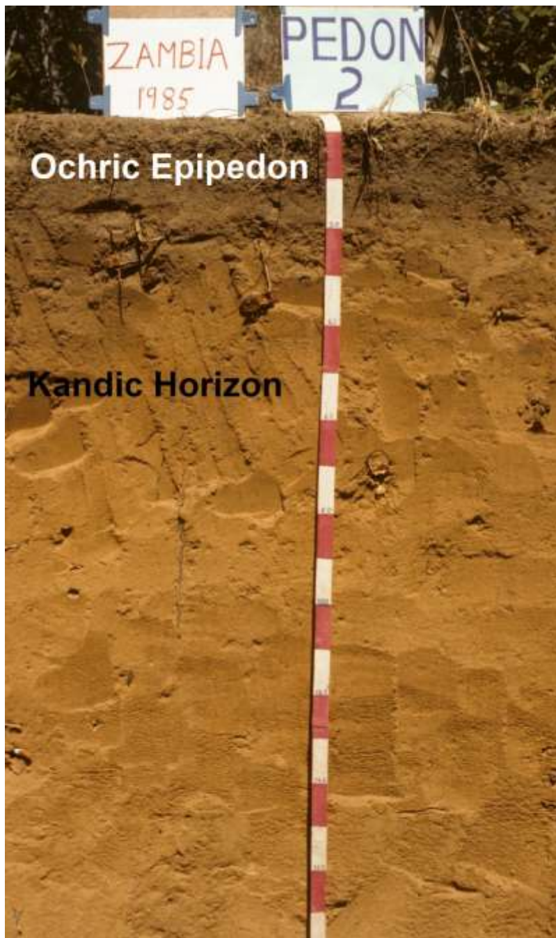
Profile of a soil in Zambia that has a kandic horizon below an ochric epipedon. Scale colors are in decimeters.
