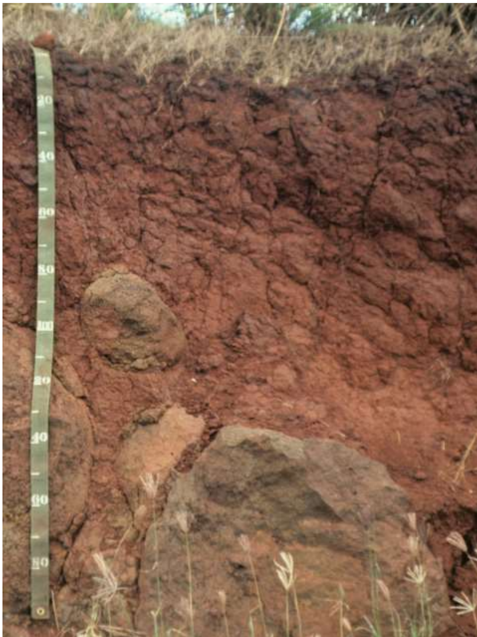
Profile of a Torrox (specifically a Haplotorrox) in Hawaii. This soil formed in colluvium containing large basalt boulders. Scale is in centimeters.
