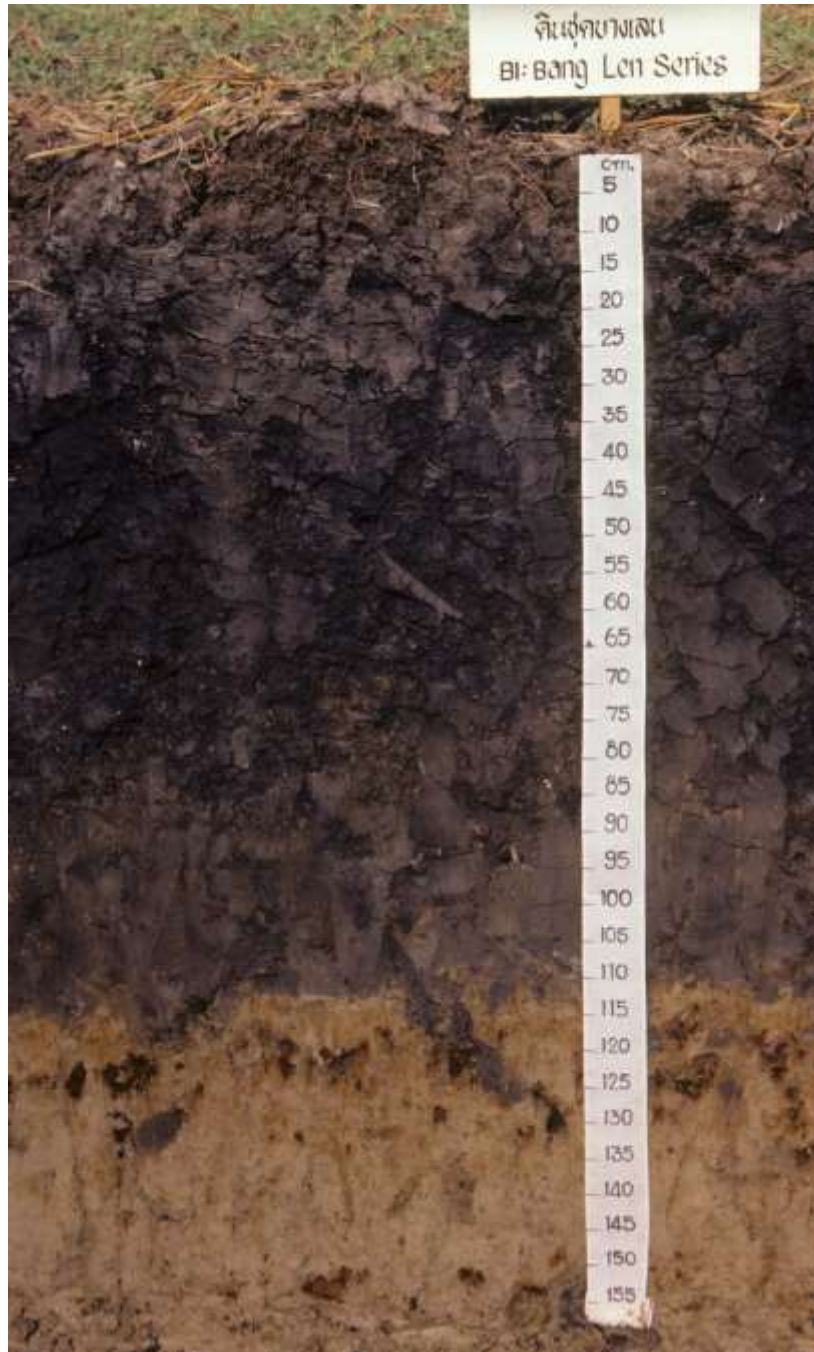
Profile of an Aquert (specifically an Endoaquert) in Thailand. Redoximorphic features are throughout the profile. A lithologic discontinuity to underlying loamy material is at a depth of about 110 centimeters. Scale is in centimeters.
