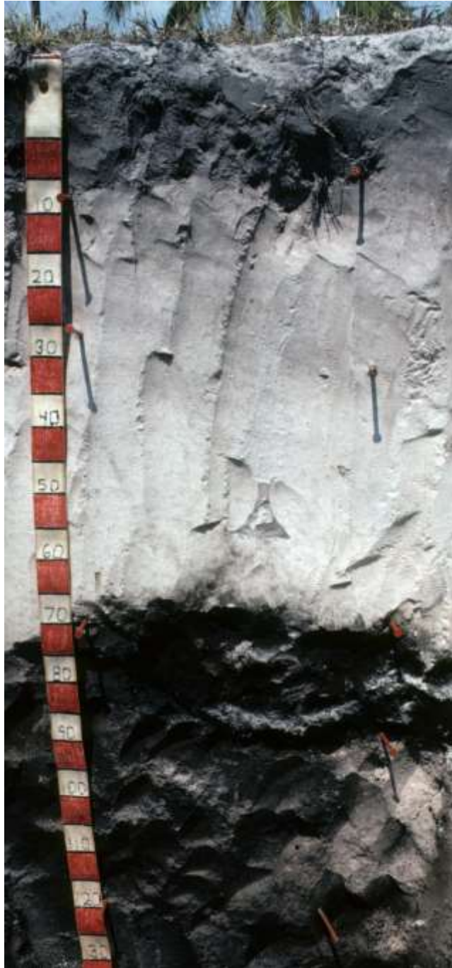
Profile of a Humod (specifically a Haplohumod). This soil has a thick albic horizon (white) underlain at a depth of about 70 cm by a spodic horizon with a high content of organic carbon. Scale is in cm.
