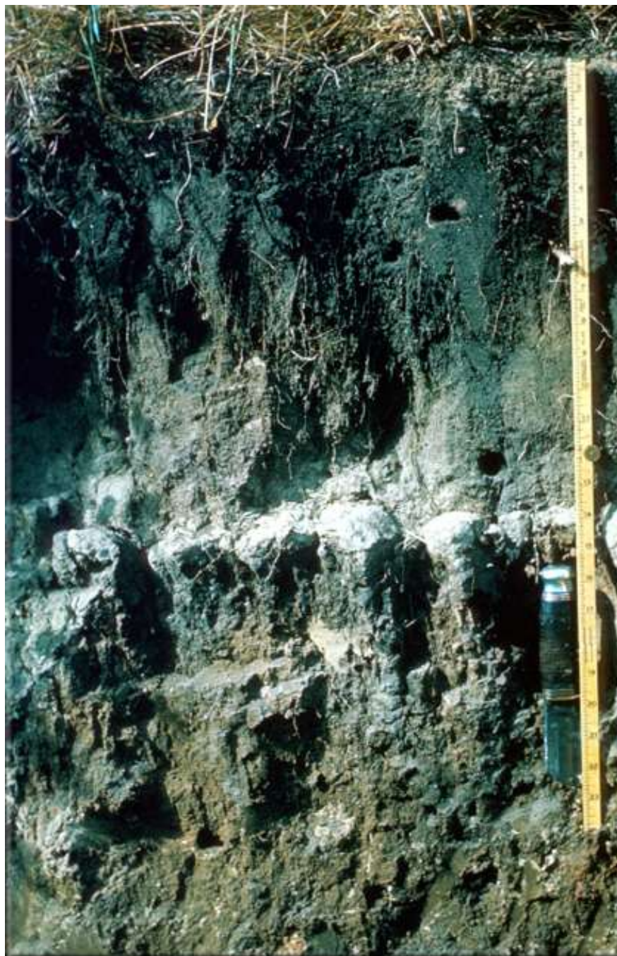
Profile of a Cryoll (specifically a Natricryoll). The soil has a natric horizon below a depth of 14 inches. Scale is in inches.
