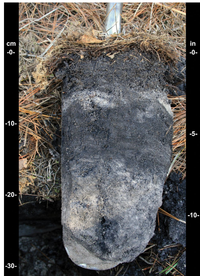
Figure 27.—Indicator S9 (Thin Dark Surface). A dark surface horizon about 5 cm thick overlies a thin layer with value of 4 or less and chroma of 1 or less. Directly below the second layer is a spodic horizon, starting at a depth of about 7 cm.
