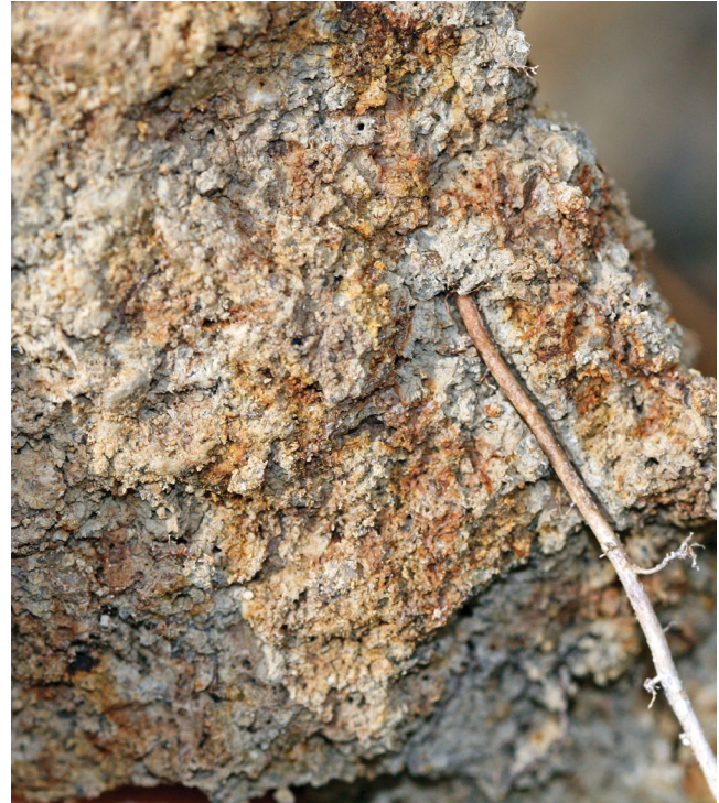
Figure 55.—Redox concentrations occurring as soft masses and pore linings. Also, a redox depletion along a root channel.
