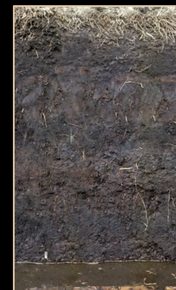
10 These soils consist of very deep organic deposits in freshwater marshes. They are in areas of flatwoods and lowlands that are very poorly drained and have a high water table. Organic materials accumulated under anaerobic conditions in areas where decomposition was very slow.
