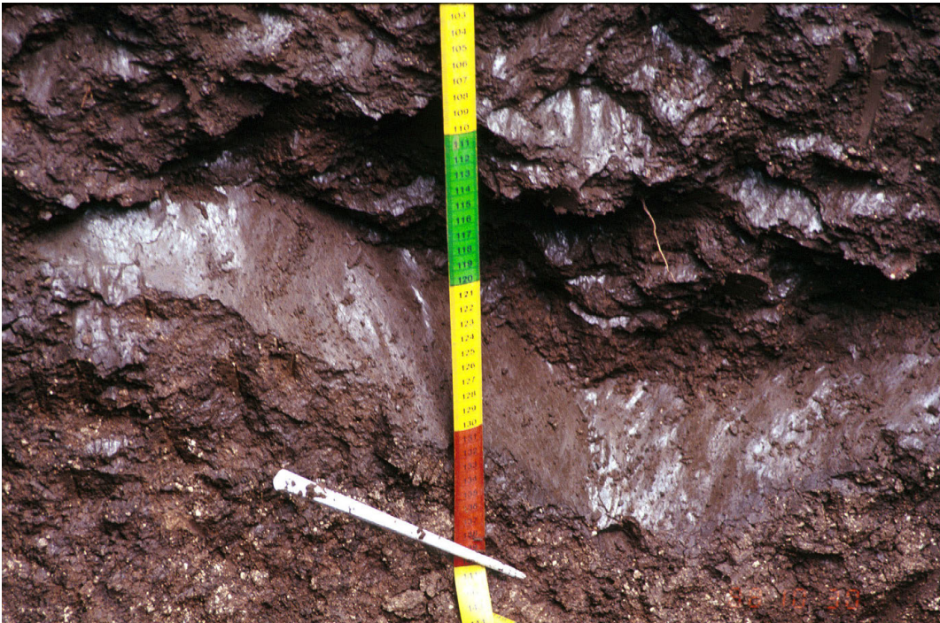
Figure 3-26: Close-up of slickensides in the lower part of a Vertisol in India. Scale is in cm.
