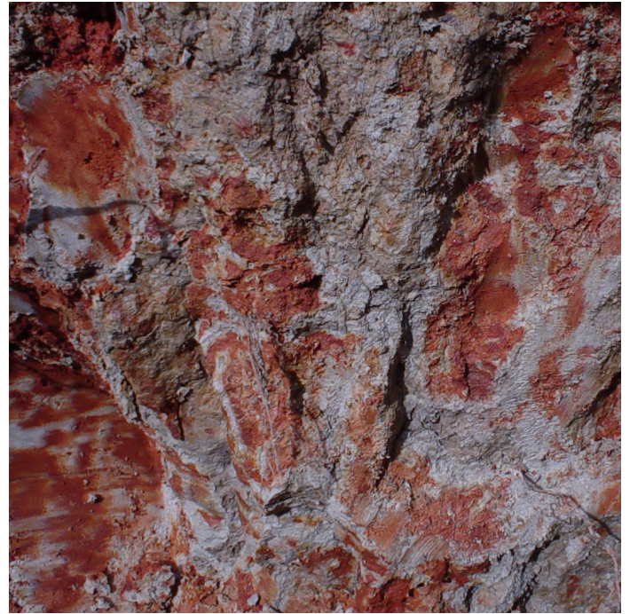
Figure 3-25: Plinthite (firm, dark red concentrations) in a soil near College Station, Texas. (Photo courtesy of Dr. David Weindorf)
