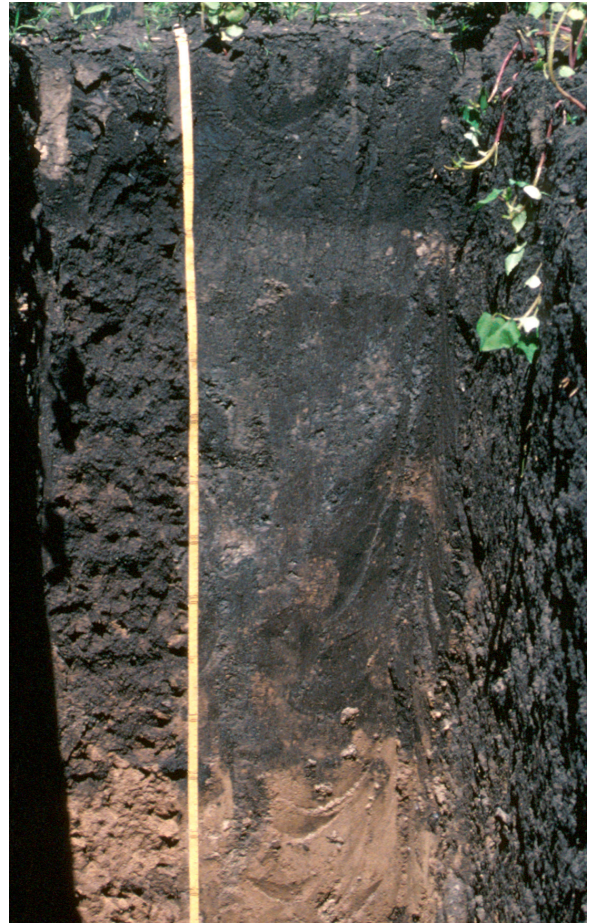
Figure 3-5: Soil with a mollic epipedon more than 1 meter thick that formed on the steppes of the Ukraine.
