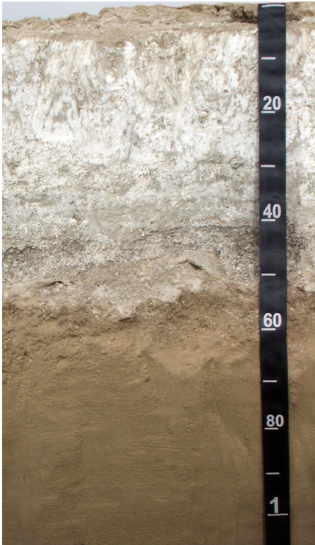
Figure 3-10: A soil profile with an anhydritic horizon (depths of 0 to 55 cm) from the United Arab Emirates. Scale is in 10-cm increments. (Photo courtesy of Dr. Shabbir A. Shahid)
