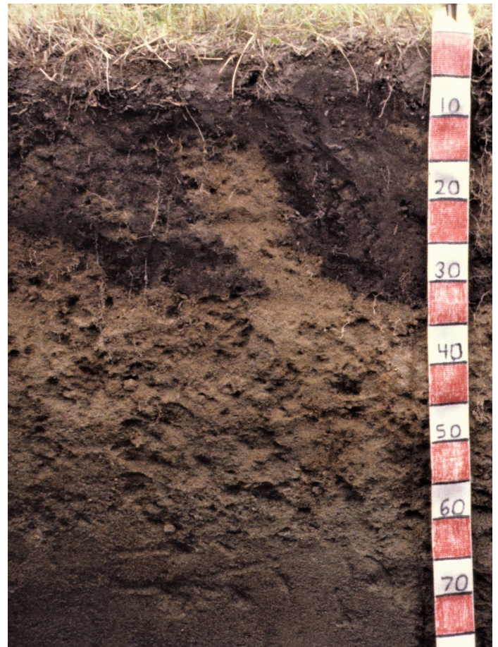
Figure 3-18: Soil profile of a Duraquod in Washington State that has a massive, horizontal, continuous ortstein layer below a depth of about 60 cm. The ortstein has been smoothed for the photo. Scale is in cm.
