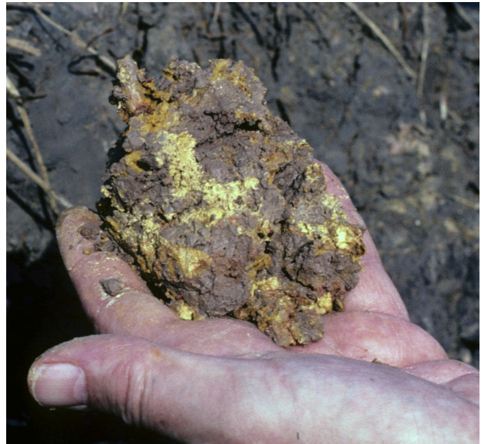
Figure 3-31: Jarosite concentrations (yellow) within peds from a sulfuric horizon.
