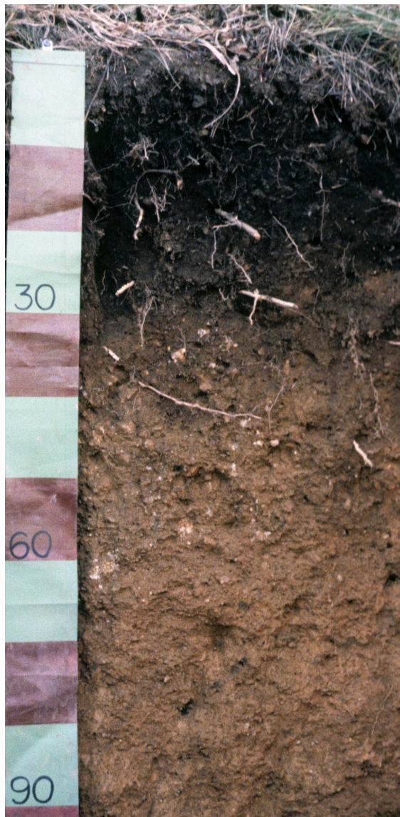
Figure 3-8: Soil profile from South Korea with an umbric epipedon about 30 cm thick. Scale colors are in 10-cm increments.
