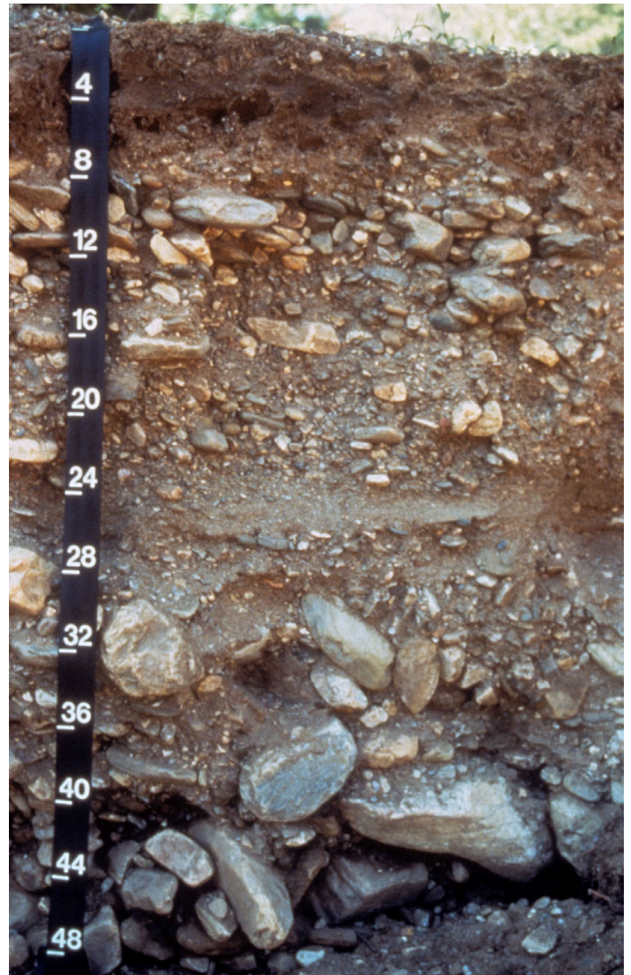
Figure 3-6: A soil profile with an ochric epipedon about 18 cm (7 inches) thick. Except for the ochric epipedon, this profile exhibits little pedogenic development. Scale is in inches.
