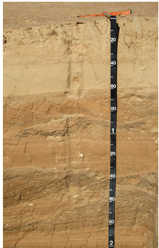
Figure 3-1: Soil profile with rock structure as fine to coarse stratifications throughout. The upper 60 cm is recent eolian sand. The lower part consists of old alluvial deposits interspersed with eolian strata. The soil is a Torriorthent in the United Arab Emirates. Scale is in cm. (Photo courtesy of Dr. Craig Ditzler)
