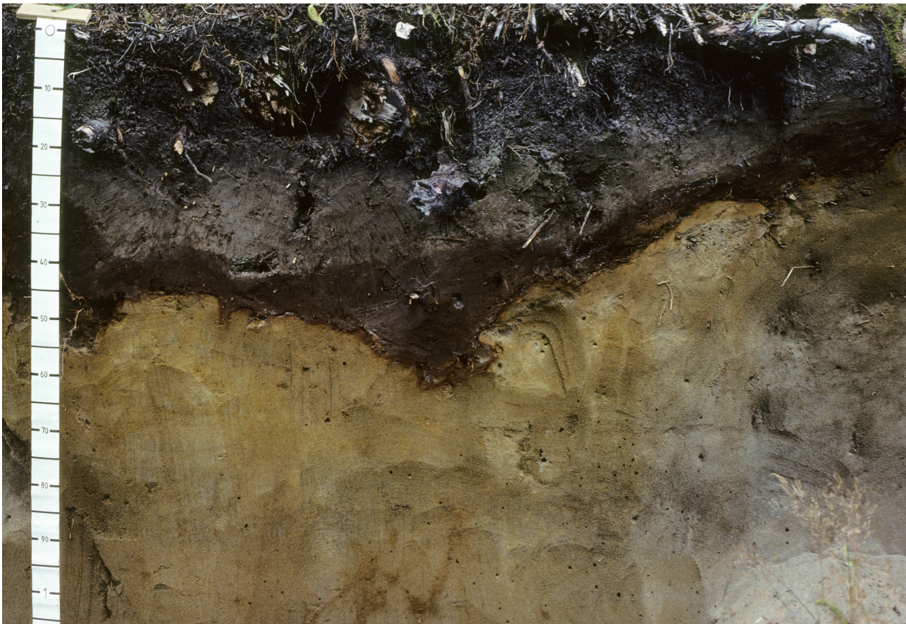
Figure 3-21: Profile of a soil in New Zealand (specifically a Placorthod) that has a thin, cemented placic horizon a few mm thick at the wavy contact between the dark yellowish brown material above and the reddish yellow material below (at a depth of about 50 cm, adjacent to the tape measure). Scale is in 5-cm increments.
