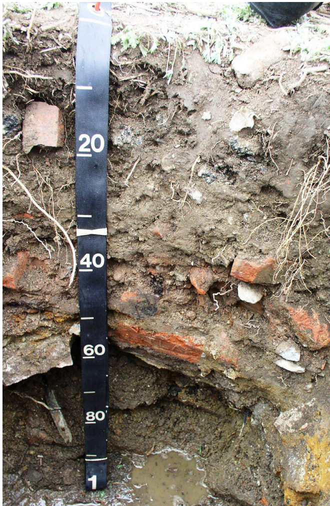
Figure 3-2: Soil profile in New York City that formed in human-transported material. It has a darkened anthropic epipedon and is rich in artifacts consisting of building materials such as brick, concrete, and metal. Scale is in cm. (Photo courtesy of Richard Shaw)
