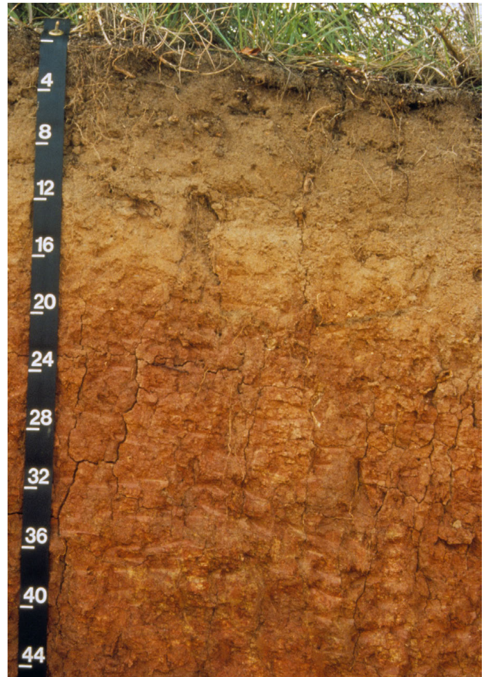
Figure 3-17: Soil profile from North Carolina with a thick, reddish yellow kandic horizon below an ochric epipedon. The kandic horizon begins at a depth of about 16 inches (41 cm) and extends below the base of the photo. The soil is a Kandiuult. Scale is in inches.
