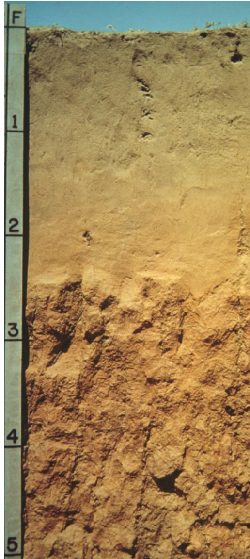
Figure 13.—Well drained Brownfield soil formed in old eolian material. Light brown fine sand (0 to 30 inches) over red and yellowish red sandy clay loam (30 to 60 inches). Arenic Aridic Paleustalf. New Mexico and Texas.
