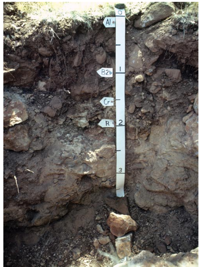
Figure 11.—Well drained Hambricht soil formed in amorphous material derived from basic igneous rocks. The content of rock fragments is about 50 percent to the Cr horizon, at a depth of 15 inches. Fractured basalt (R horizon) is at a depth of 19 inches. Lithic Haploxeroll. California.
