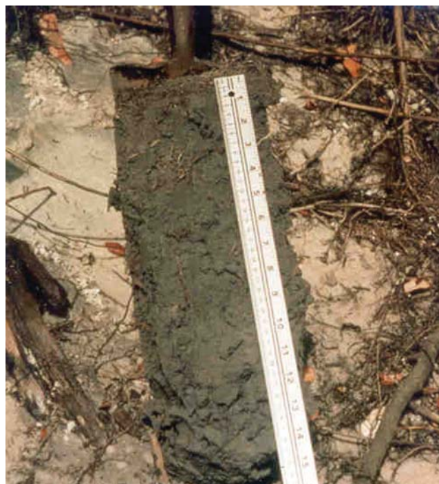
Figure 20.—Indicator S4 (Sandy Gleyed Matrix). The gleyed matrix begins at the soil surface. Scale is in inches (R) and cm (L).
