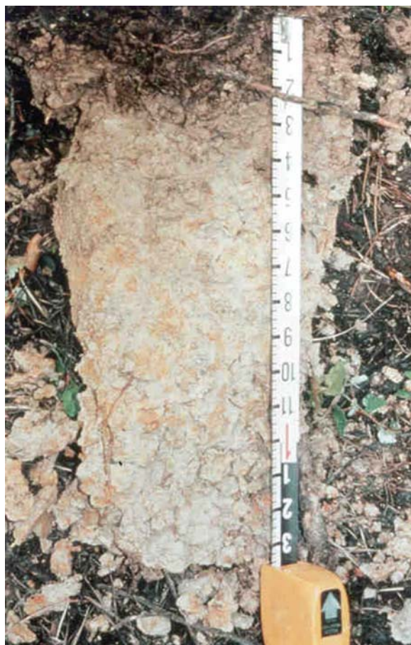
Figure 29.—Indicator F3 (Depleted Matrix). Chroma is 2 below a depth of about 15 cm. Redox concentrations are present. Scale is in inches.
