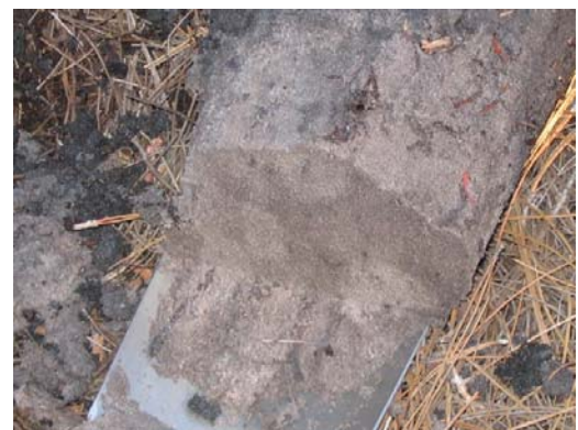
Figure 24.—A soil that does not meet the requirements for Indicator S6 (Stripped Matrix) because the splotches are distinct rather than diffuse.
