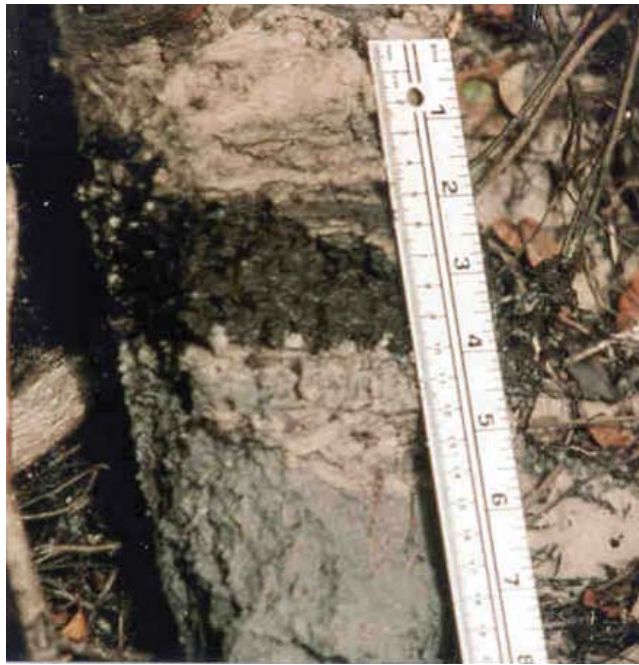
Figure 11.—Indicator A5 (Stratified Layers) in loamy material. Scale is in inches (R) and cm (L).
