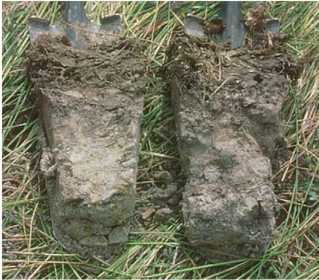
Figure 44.—The profile on the right is from a drained wetland adjacent to a ditch. The profile on the left is from an area not affected by the ditch. Both soils meet the requirements for indicators F3 (Depleted Matrix) and A11 (Depleted Below Dark Surface) and thus are hydric soils.
