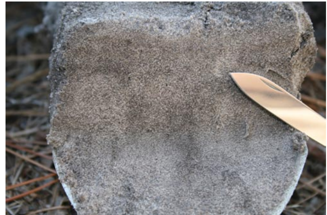
Figure 24.—Indicator S6 (Stripped Matrix). This indicator requires diffuse splotchy patterns with rounded areas stripped of organic matter or iron, as exemplified in this photo.
