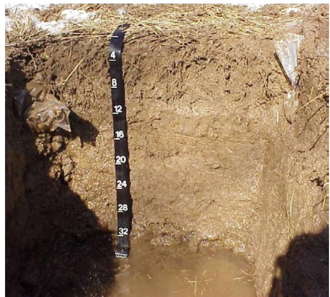
Figure 42.—Indicator F3 (Depleted Matrix) in red parent material. If a soil that formed in red parent material stays wet and anaerobic long enough, it may develop the indicator F3.
