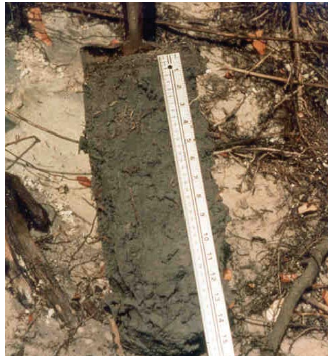
Figure 21.—Indicator S4 (Sandy Gleyed Matrix). The gleyed matrix begins at the surface of the soil.
