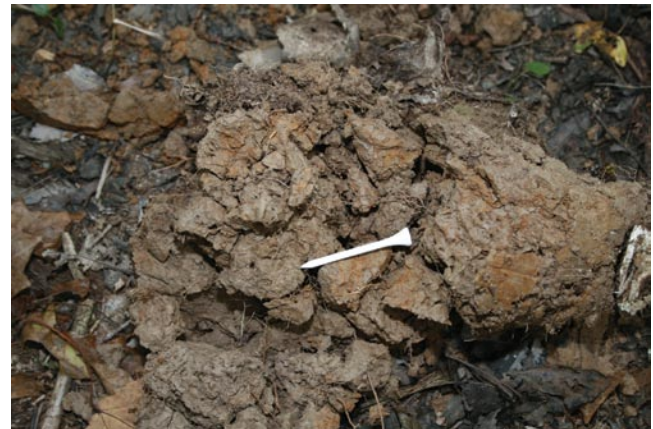
Figure 37.—Indicator F12 (Iron-Manganese Masses). While this indicator requires only 40 percent value of 4 or more and chroma of 2 or less, at least 2 percent iron-manganese masses is needed. These masses are indicated by black splotches in this photo.
