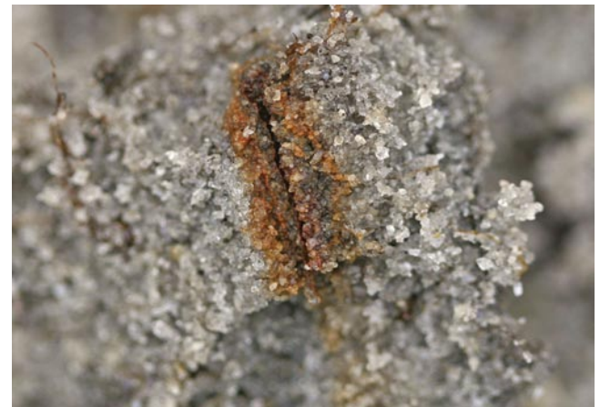
Figure 54.—A redox concentration occurring as a pore lining.
