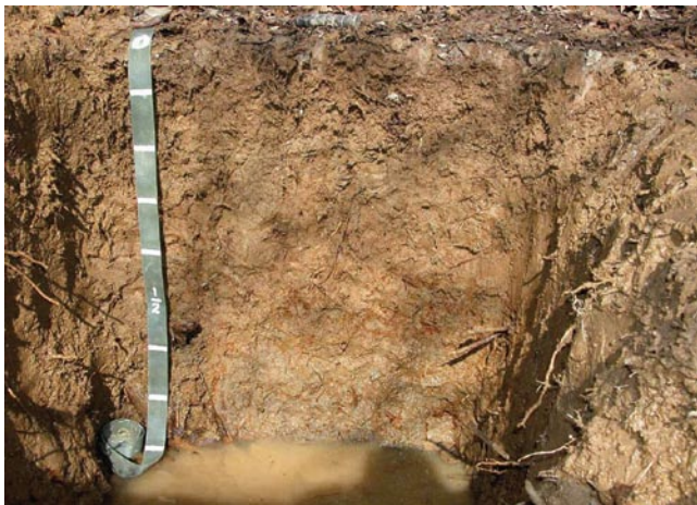
Figure 39.—Indicator F19 (Piedmont Flood Plain Soils). This indicator is restricted to active flood plains. It does not require a matrix color with chroma of 2 or less.
