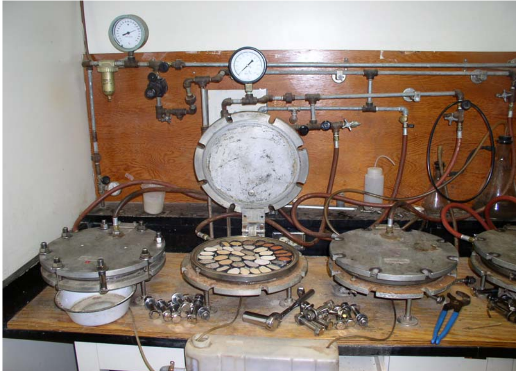
Figure 1. Sieved (<2-mm) soil placed in pressure-membrane extractor.
