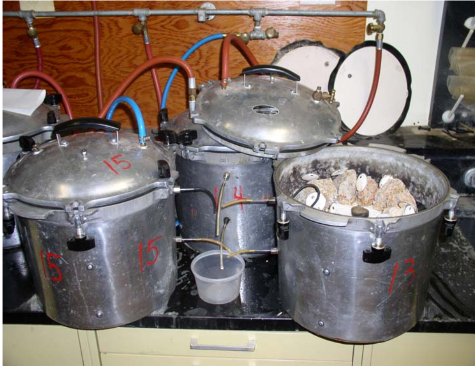
Fig 1. Clods placed in pressure-plate extractor following saturation.
