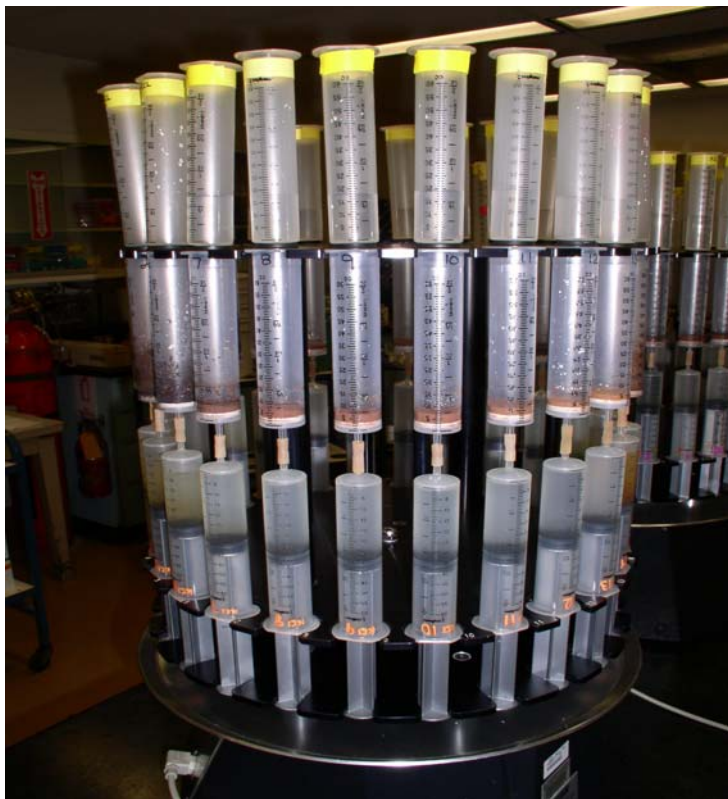
Fig.1. Mechanical vacuum extractor, SAMPLETEX, MAVCO Industries, Lincoln, NE.
