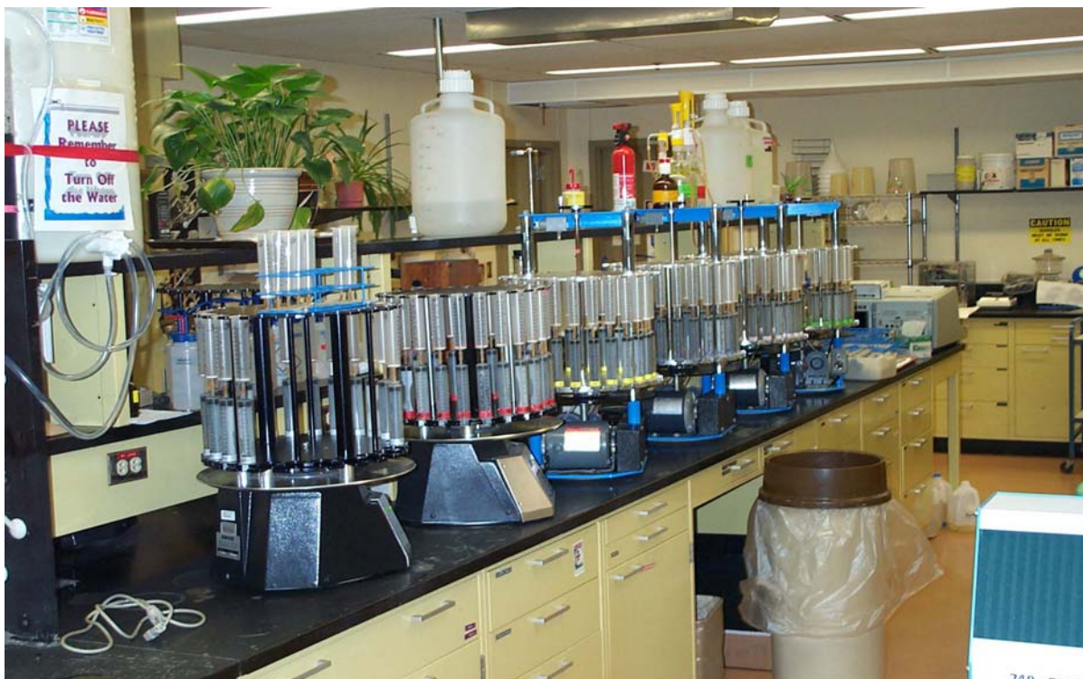
Fig. 2. Mechanical vacuum extractor used at the USDA-NRCS Soil Survey Laboratory for chemical extractions and analyses, e.g., cation exchange capacity, \text{NH}_4\text{OAc} , pH 7.
