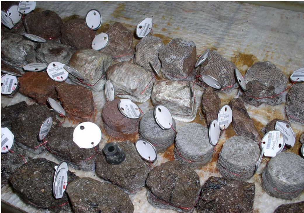
Fig. 2. After a flat surface on the clod is cut with a diamond saw, the clod is placed on a tension table, maintained at 5-cm tension.
