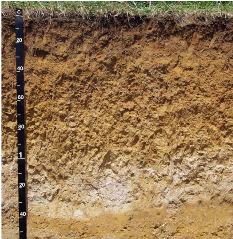
Fig. 3. Photographs are typically taken of soil profile after the layers have been identified but before the vertical section by the sampling process.
