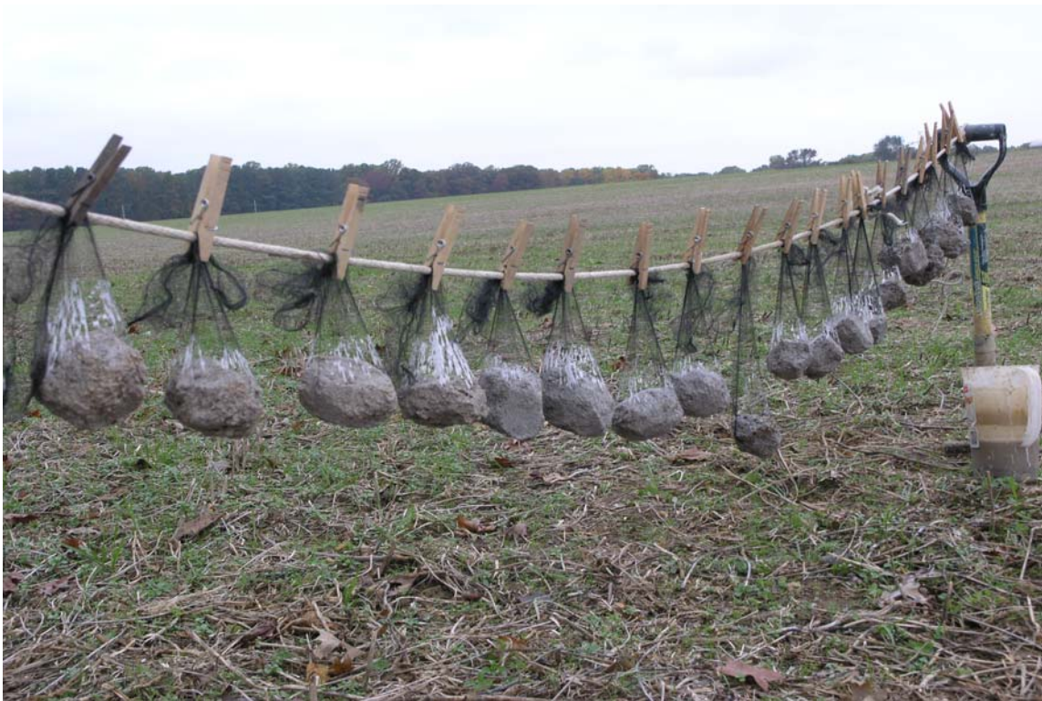
Fig. 2. After dipping, clods are tied to clothesline to dry.
