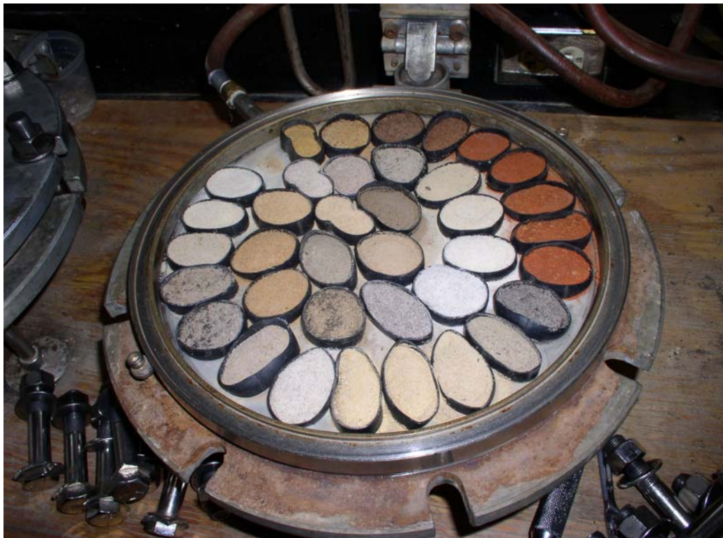
Figure 2. Pressure-membrane extraction at 1500-kPa for <2-mm samples.
