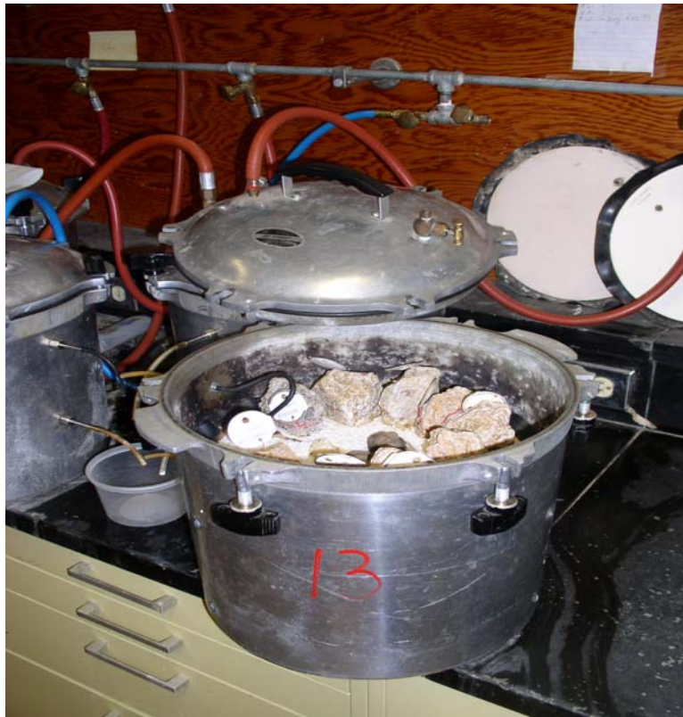
Fig. 2. Pressure-plate extraction at 33-kPa for clods.
