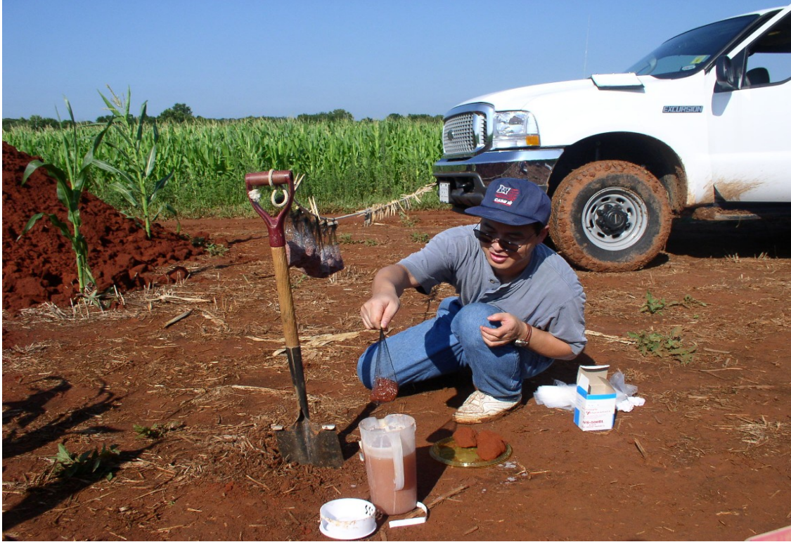
Fig. 1. Dipping clods with hairnet in plastic-lacquer.
