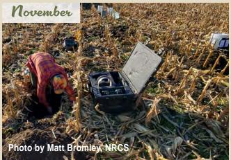
**Saturated hydraulic conductivity** (Ksat) is a quantitative measure of the ability of a saturated soil to transmit water when subjected to a hydraulic gradient. In Pulaski County, Indiana, soil scientists measure Ksat with an infiltrometer to understand the link between soil properties, climate, and management type. This site is within the Kankakee River Basin, where the Grand Kankakee Marsh once stretched.
